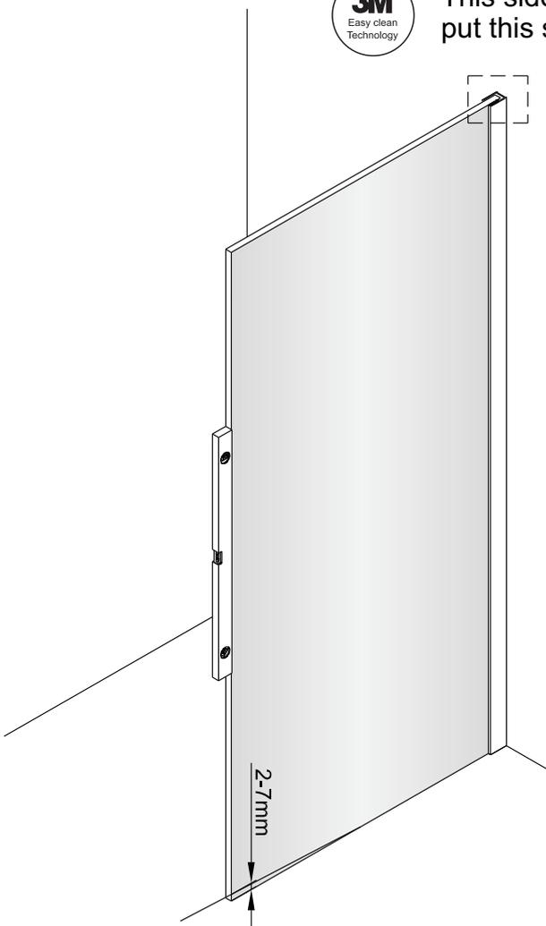
When the bottom fixed door is not in line with the floor or tray edge, the setting wedge 7 will be needed and can pad 2-7mm.
